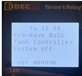
Press DOWN arrow then ESC. “Program” should be highlighted. If not, use up and down arrows keys to highlight “program”.
